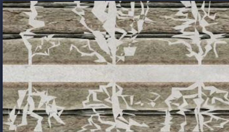
After perforation and subsequent hydraulic fracturing
