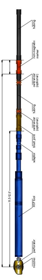
Underground hydro-slotting perforation tool for vertical wells (Patent **US 8863823**) is consists of perforator with jet's nozzles, return block, hydraulic block, shank, and adaptor (picture on the left).
